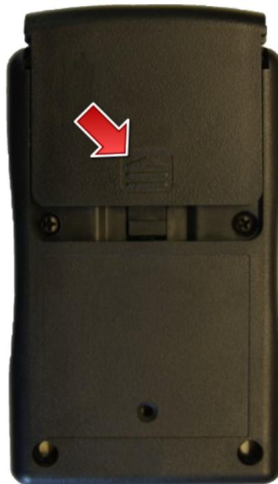
Fig. TachoReader Combo - battery change.
